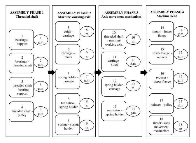
Fig. 2 - Graphical representation of the workstations of the overall assembly of machine head with indication of the specific type of performed controls. Legend of the type of control: g: geometric, m: mechanical, d: dimensional.
