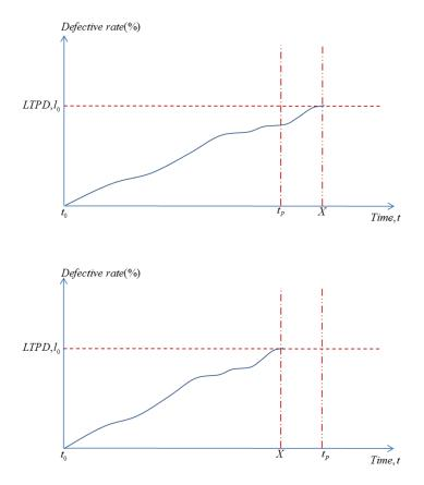
Figure 1 – Defective rate with optimal manufacturing quantity and LTPD: manufacturing process should be checked at earlier time between the shifted time *X* from *in-control* condition to *out-of-control* condition and optimal manufacturing quantity time  $t_p$
