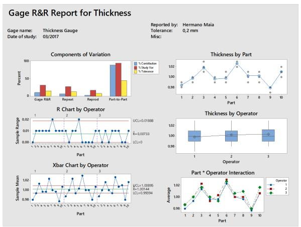
Figure 20 - R&R test applied to the thickness gauge
