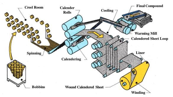
Figure 14 – Calendering line of metallic material
