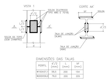
Figure 4 – Detail of splicing of steel piles. Source: Foundation project (2015)
