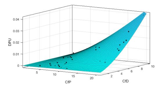
Fig. 3 - 3D surface plot of DPU against  $Cf_P$  and  $Cf_D$ . (experimental points of 30 workstations concerning an analogous assembly process for mechatronic devices, and theoretical model)
