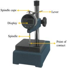
Figure 16 – Thickness Gauge
