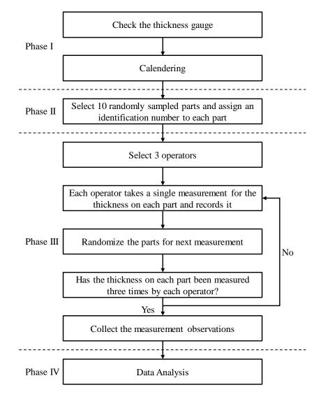
Figure 19 – Procedure of the R&R test applied to the thickness gauge
