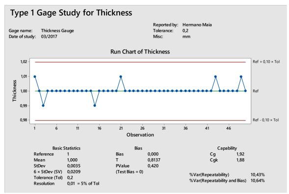
Figure 18 – Type 1 study for thickness
