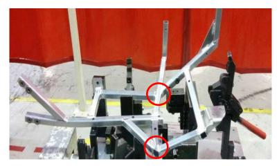
Figure 3 – Welding operation no. 30. Red circles show the corresponding weld areas.
